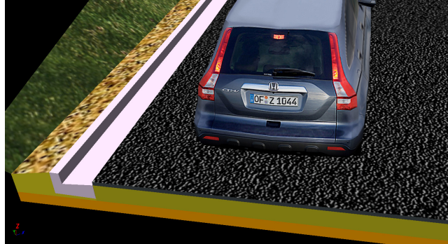
Kerbs, pavement, material courses etc as digital data (strings, trimeshes etc) in 12d Model
