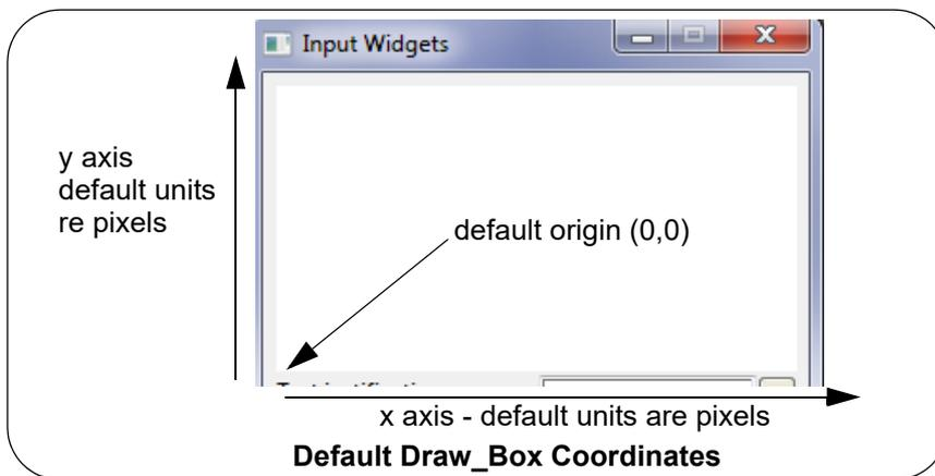
The coordinates of the bottom left hand corner can be modified by a *Set\_origin* call (see [\\_Set\\_origin\(Draw\\_Box box,Real x,Real y\)](#)), and the units for the x-axis and the y-axis can be scaled by a *Set\_scale* call (see [\\_Set\\_scale\(Draw\\_Box box,Real xs,Real ys\)](#)).
