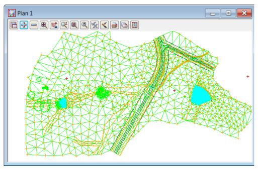
The triangles around the edge of the data have been partially nulled by the Triangulation function but we need to trim the triangles even further to be able to create a boundary around the edge of the survey.
