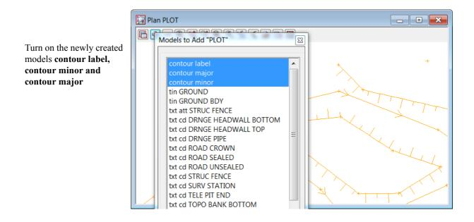
The major contour appear to be crossing the labels. This is because the model contour label was turned on prior to the other contour labels. This can be rectified by moving the contour label model to the top of the model list
