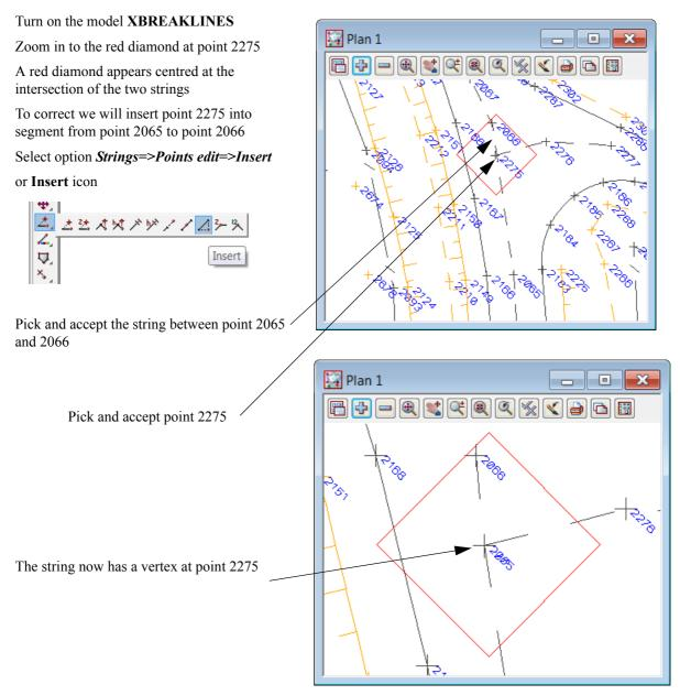
Lastly delete the diamond string surrounding the crossing breakline. We delete the diamond string as it has levels at the vertices and if the *Check Breakline* option is rerun without the **Clean models** option ticked, more crossing breaklines would result
