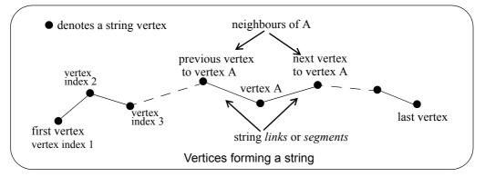
Strings vary in complexity from 2d (x,y and constant z value) to multidimensional, and an alignment string that has both horizontal and vertical geometry independently defined.
