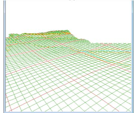
The effect of the creeks superimposed on the TIN (shown above) is created by turning on the Drainage models. Click LB on the + sign button in the View Button Area and double click LB on **survey TOPO BANK BOTTOM**, **survey TOPO BANK TOP** and **survey TOPO DRAIN** CL.
