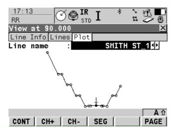
On board the Leica the strings are cut at the required chainage and a section can be viewed
