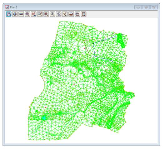
Note that the TIN is clipped at the selected **Null polygon** ensuring only the surveyed data is included. Now that we have a TIN we can display the TIN data in a variety of ways.
