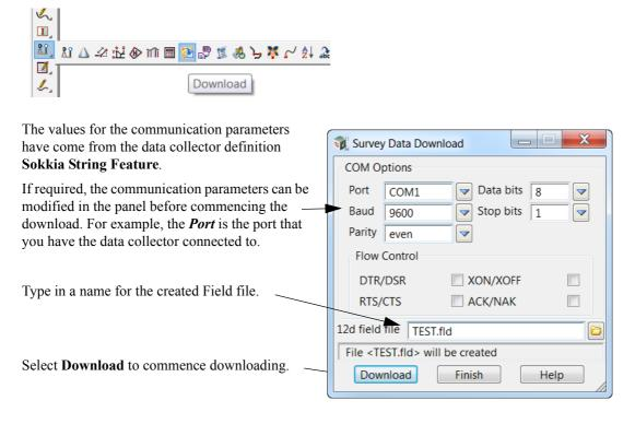
NOTE - you must have a data collector attached to the nominated COM port to be able to download data The **Comms Capture** panel is automatically placed on the screen to display messages for the download.
