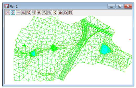
The triangulation is shown with preliminary nulling around the edge
