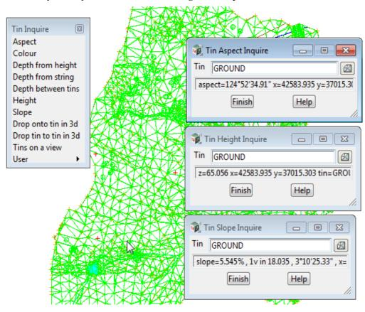
Once all three panels are on the screen, move the cursor anywhere over the TIN and observe what happens. When the cursor is positioned over any one triangle, the three point coordinates of the triangle are being used to linearly interpolate *on the fly* to calculate the exact x,y,z coordinates of the cursor. Also the aspect and slope of the triangle is shown in the respective panels.
