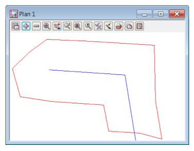
To insert a curve into the centreline string select option *Cad* =>*String* =>*Join fillet*
