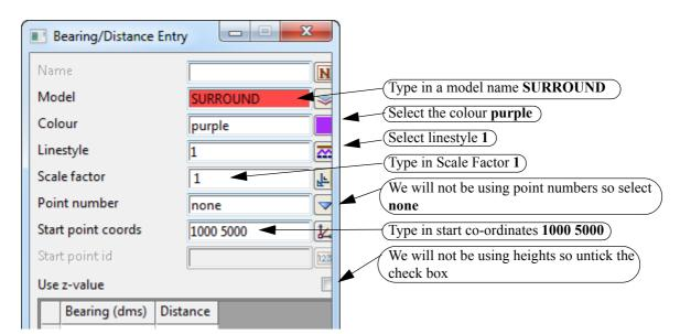
We are now able to type in the bearing and distances around the edge of the boundary
