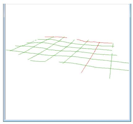
The appearance of the mesh can be improved by reducing the mesh spacing.
